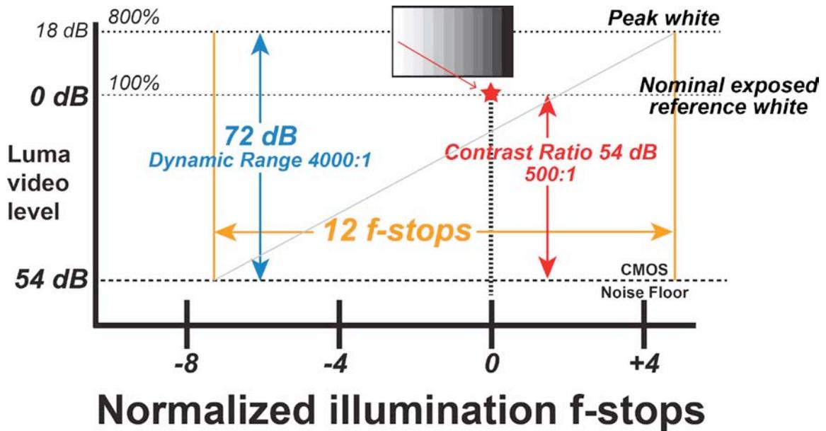
**Figure 15** Showing the deployment of the potential matrixed Luma 72 dB of total dynamic range between a 54 dB contrast ratio (for the nominally exposed signal portion) and the remaining 18 dB range for dealing with over-exposed portions — when camera Master Gain is set to 0 dB
