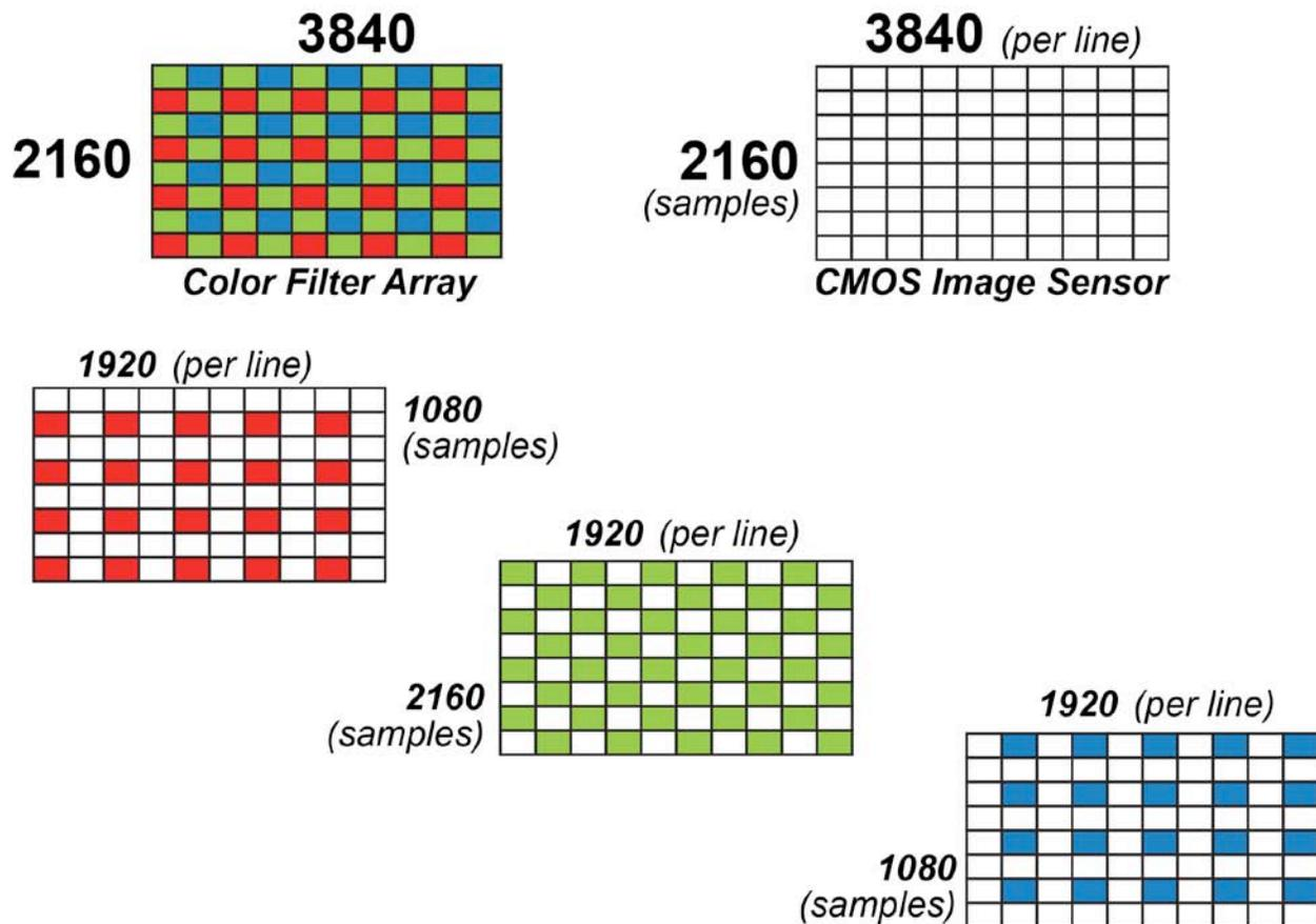
**Figure 4** *Illustrating the separate CFA array and the CMOS imager while also showing the CFA separated into its component color filters to better expose the structure of their respective sparsely-sampled lattices*
