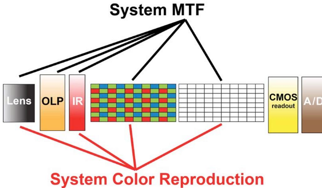
**Figure 2** Showing the essential system elements that constitute the image sensor system and the external optical elements (lens, optical low pass filter, IR filter) that precede the sensor in the Canon EOS C300 digital cinema camera — and their collective bearing on some key performance parameters
