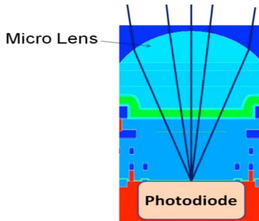
*Figure 3* Showing a cross-section of a single photosite
